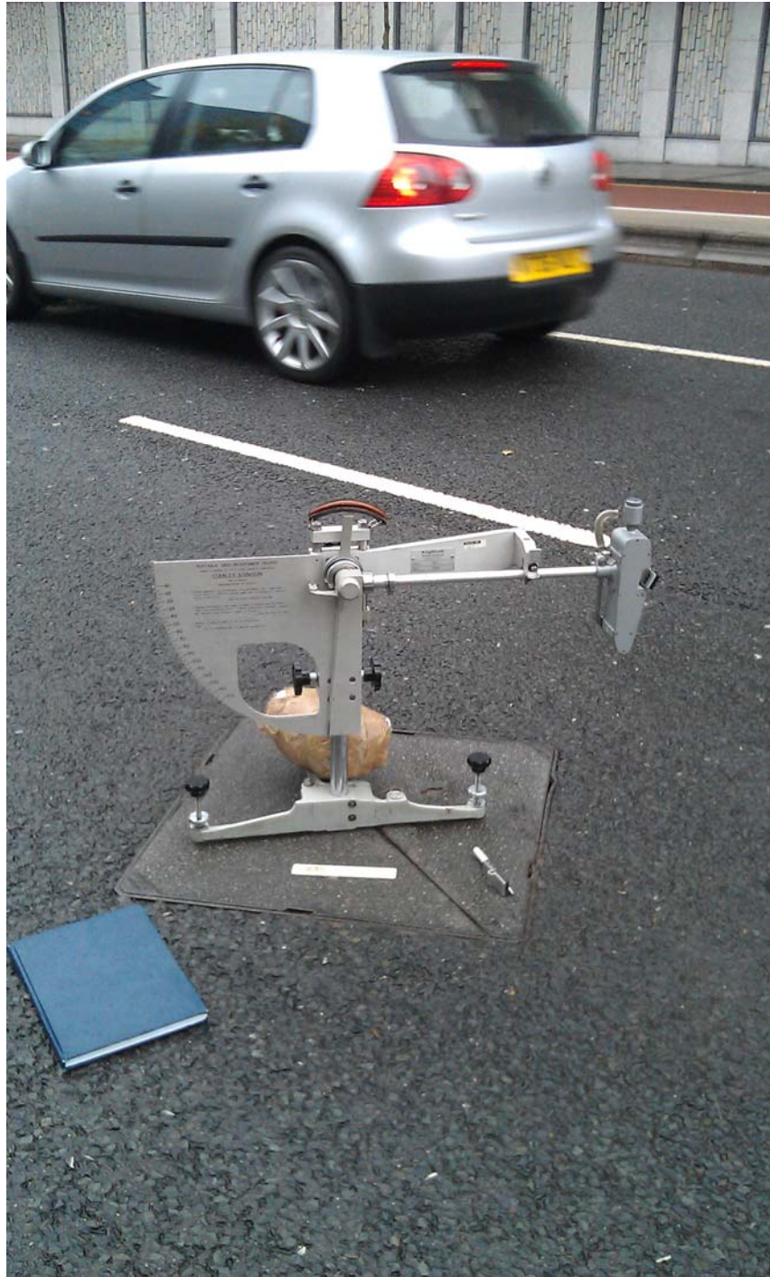
Example of Test Location
